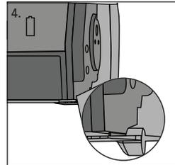
4. Bottom of module side walls should be parallel to and flush with bottom of housing.
