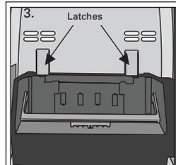
3. Push module straight down ensuring both latches engage fully.
