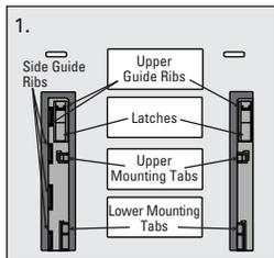
1. Identify attachment components in housing.
