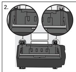
2. Locate upper rear surface of module side wall against upper guide ribs in housing. Left rear side wall of module should be in contact with side guide ribs and module fully seated and flat against back of housing brackets.
