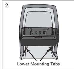
2. Position top of module side walls at top of recess. Module should be above lower mounting tabs and fully seated and flat against back of housing.
